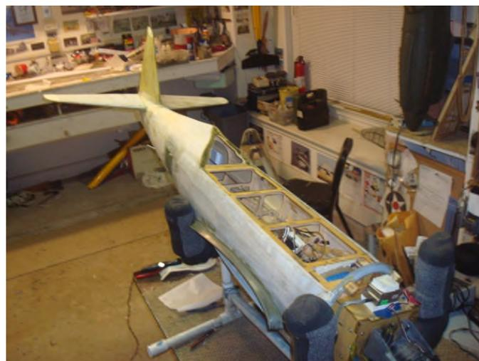
I glassed the wood areas using silk sheet and finishing resin. Coverite on the control surfaces. The wings and fuselage were sanded with light sand cloth. The panel lines were applied with 1/16" chart tape, referenced from a P47 three view. Then two coats of dry sandable primer were applied. The chart tape was removed 24 hours later to reveal the panel lines.
